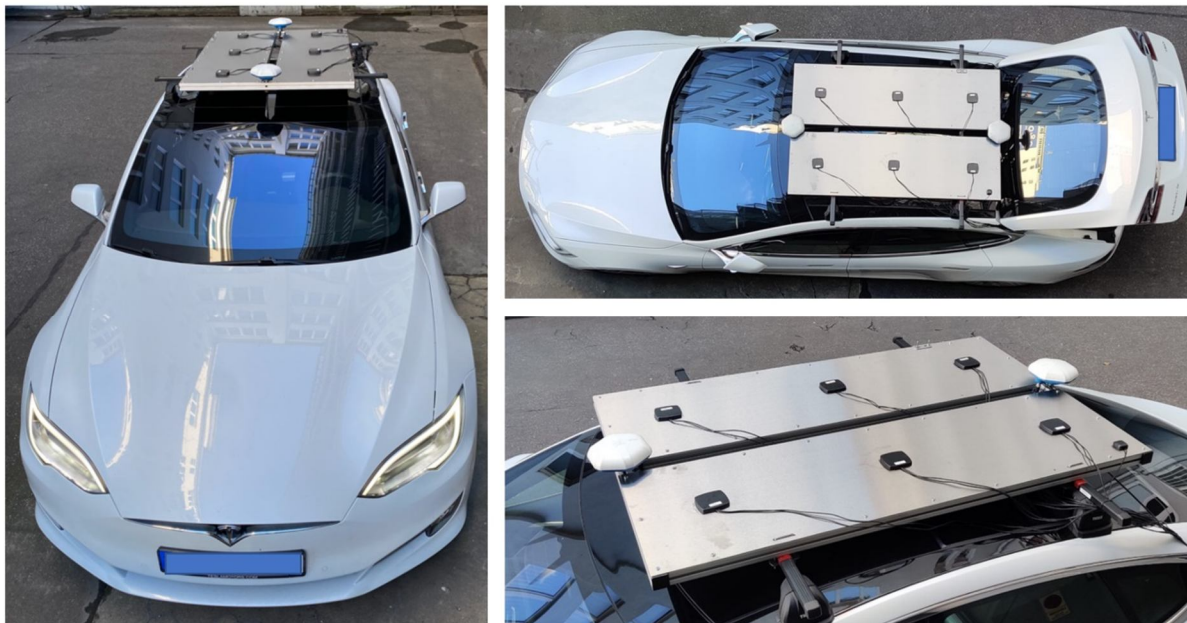
Figure 1. The antenna setup of the vehicle.
