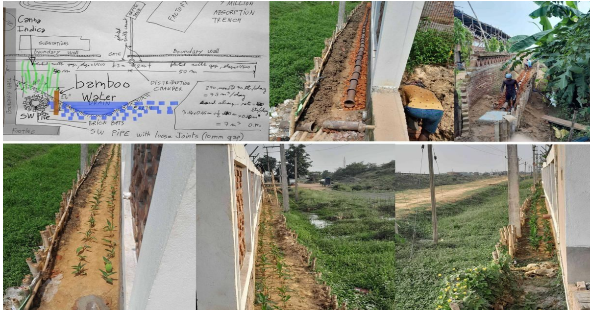
Fig. 4 The sketch diagram of the Rootzone treatment
