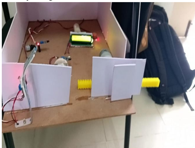
Fig. 5. Vehicle number plate recognition and gate opening
