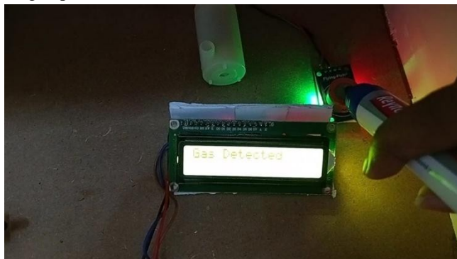
Fig. 12. Gas leakage detection and warning system
