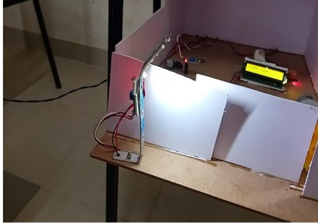
Fig. 10. Automatic street light control based on day/night detection
