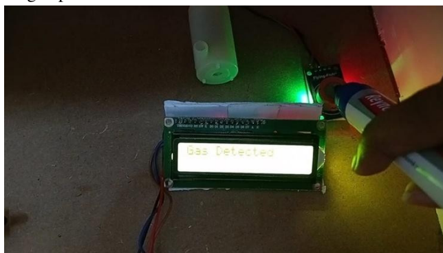
Fig. 12. Gas leakage detection and warning system
