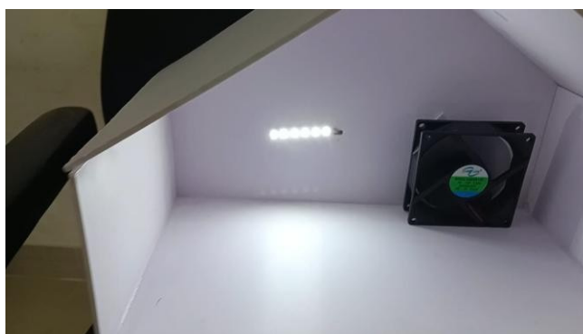
Fig. 11. Indoor light and fan automation when person enters home
