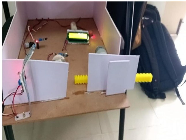
Fig. 5. Vehicle number plate recognition and gate opening
