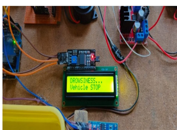
Figure 6 & 7: Checking the Drowsiness Detection; If detected the Motor Slowdown and After Sometime Vehicle Stop
