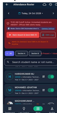
Fig. 6 Student Attendance Roster & Multi-Provider Cloud SMS Gateway: Automated absentee dispatching via Fast2SMS and Twilio webhooks.
