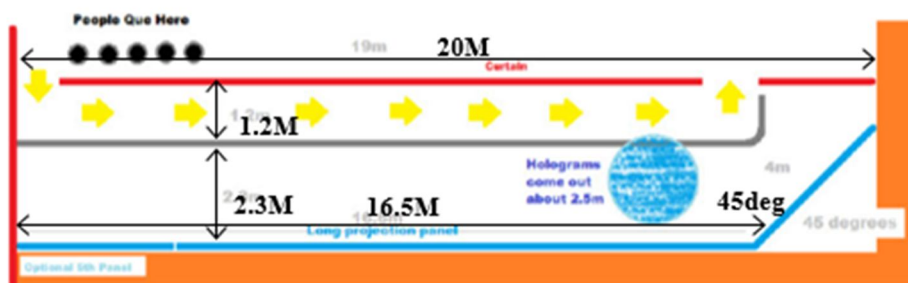
Fig. 5 Schematic plan of Hologram Tunnel
