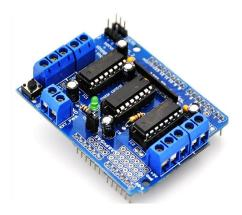
L293D is a typical Motor driver or Motor Driver IC which allows a DC motor to drive in either direction. The L293D is a 16-pin Motor Driver IC which can control a set of two DC motors simultaneously in any direction. The L293D is designed to provide bidirectional drive currents of up to 600 mA (per channel) at voltages from 4.5 V to 36 V (at pin 8!). You can use it to control small dc motors - toy motors. Sometimes it can be extremely hot.
