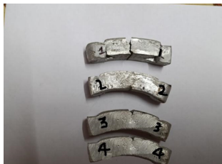
Fig.21 Samples after performing Charpy Impact test
