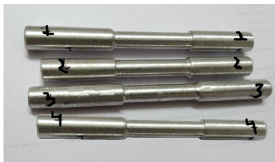
Fig.14 Tensile test machined specimen
