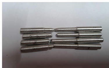
Fig.15 Samples after Tensile test
