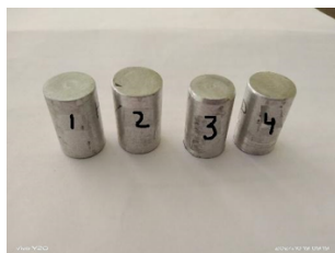
Fig.18 Machined specimen for hardness test
