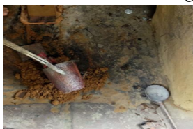
Fig.9 Pouring the liquid metal into mould
