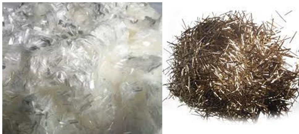
Figure 1: Pictures of PVA fiber and basalt fiber.
