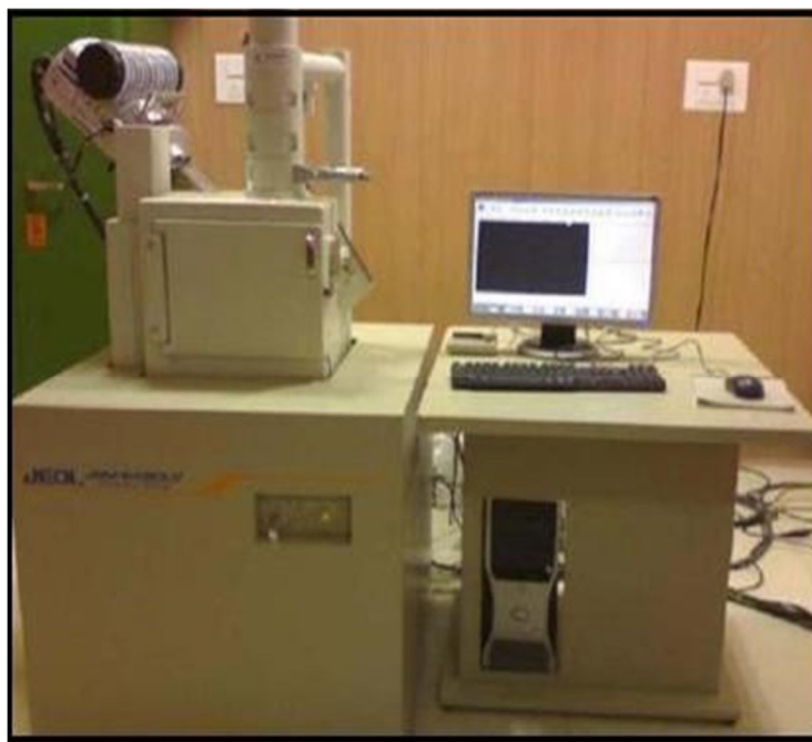
Fig. 3.4 Scanning Electron Microscopy (JEOL JSM-6480LV)
