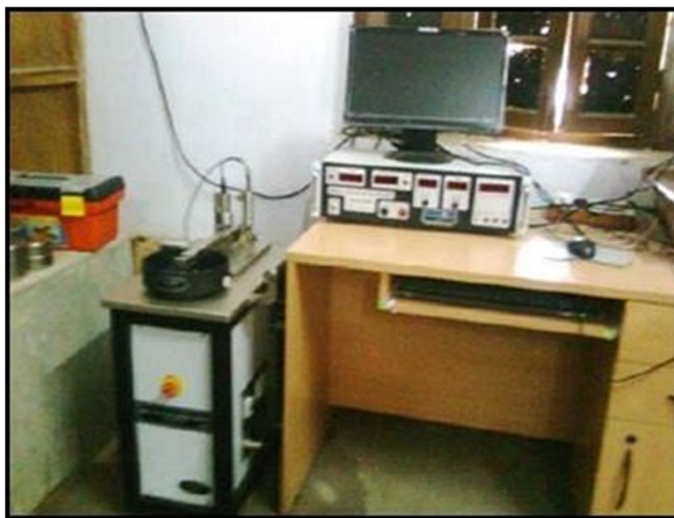
Fig.3.2- Ball-On-Plate Wear Tester (TR-208 M1)
