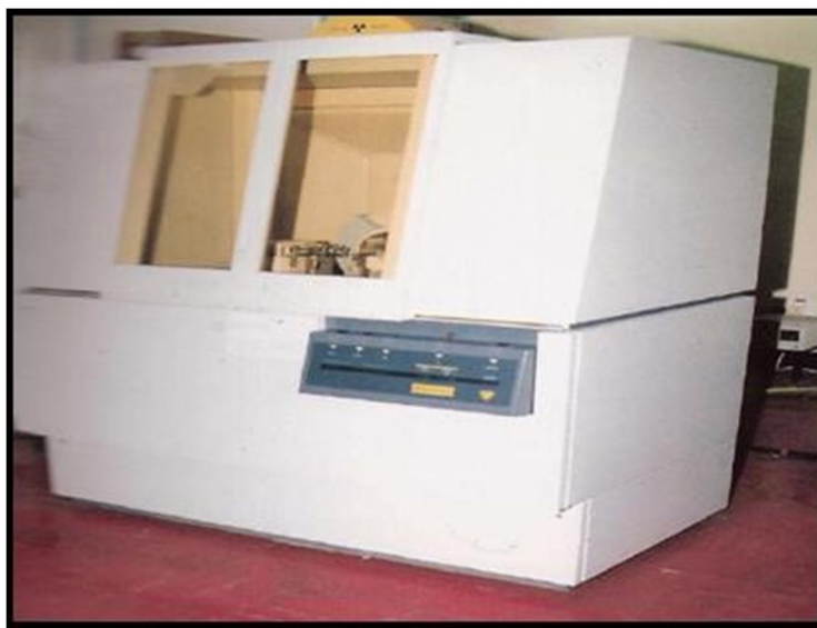
Fig.3.5 Philips X-pert multipurpose x-ray diffractometer
