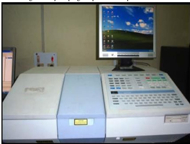
Fig.3.6 Perkin-Elmer Spectrum RXI, (FTIR) Spectrometer
