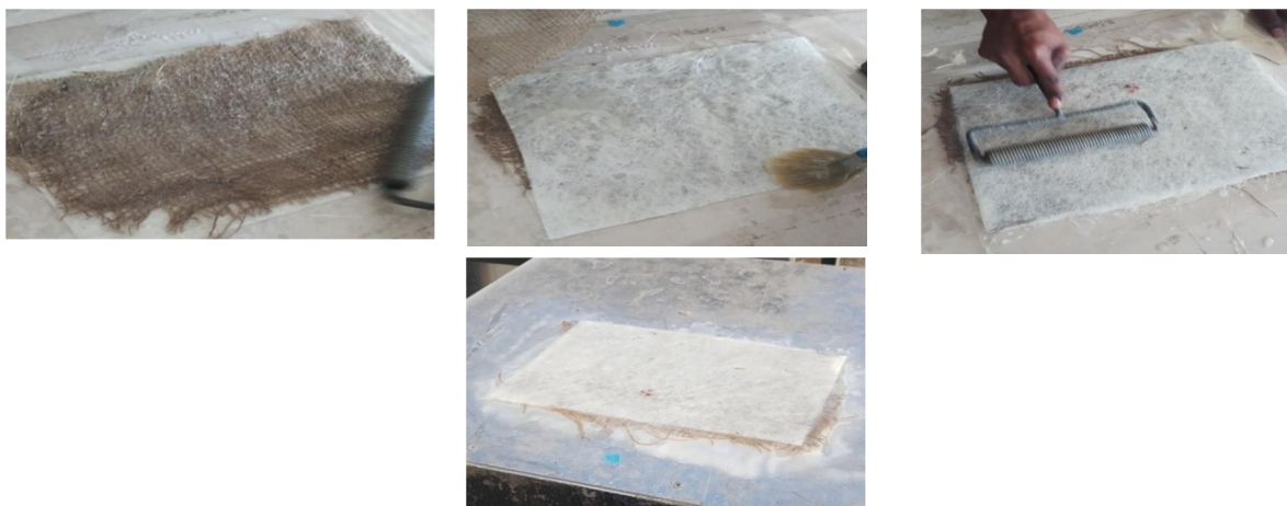
Figure 7. Fabrication by Hand-Lay Up Process
