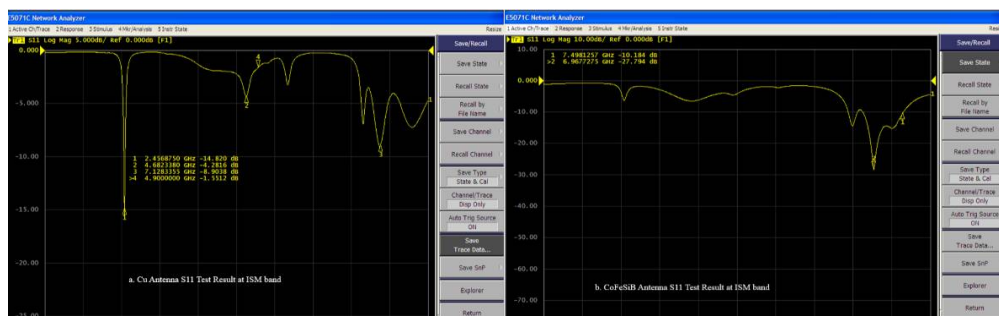
Figure 5 Antennas Test Results at ISM Band
