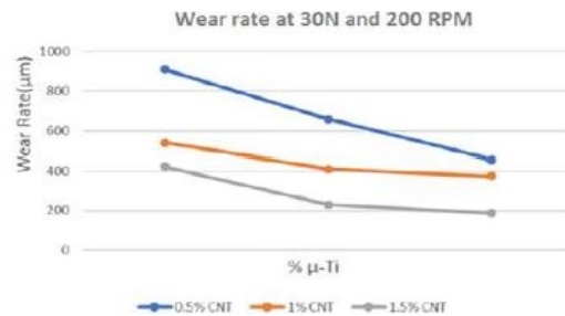
Figure 5.9 Wear rate of copper hybrid metal matrix composites at 30N & 200 RPM
