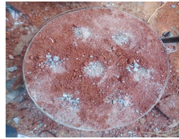
Figure.3: Soil with stone column arrangement
