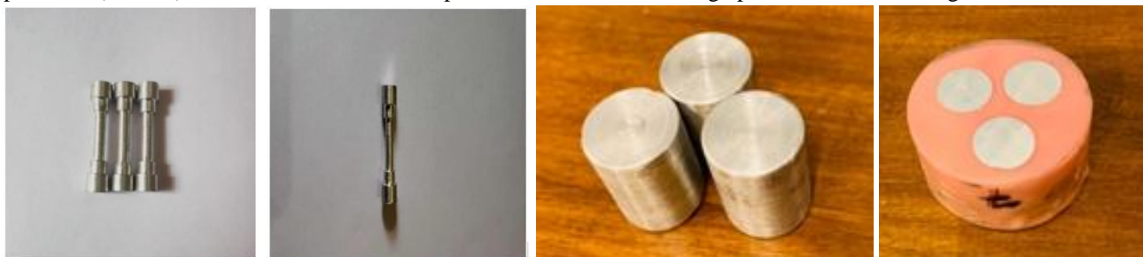
Figure 8: Specimen Preparation as per ASTM standard dimensions
