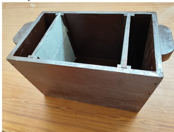
Fig. 1. Fabricated Plywood Test Box
