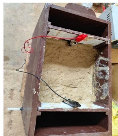
b. Model box filled with soil, Anode and Cathode electrodes connection.
