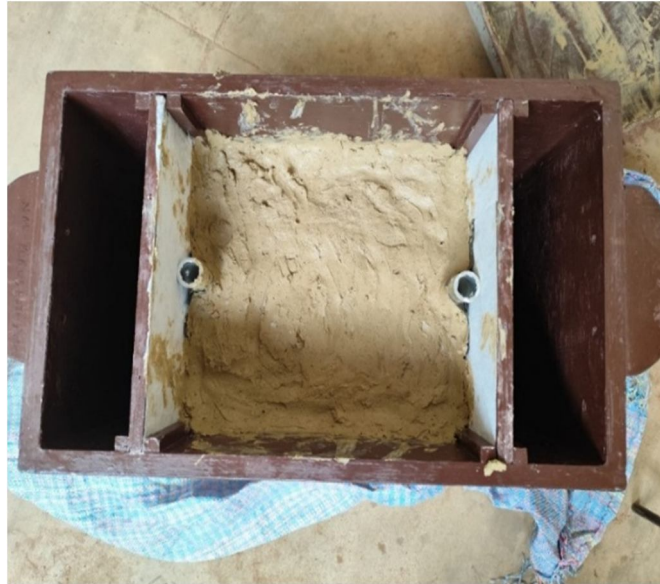
Fig. 3. Arrangement of soil samples and electrodes in the model box.
