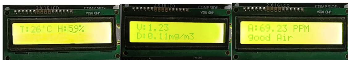
Fig.4. Displays showing Output of Temperature And Humidity, dust and gas sensors
