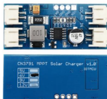
Fig.8. MPPT (Maximum Power Point Tracker)
