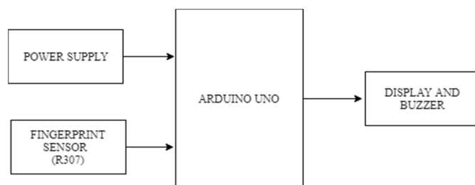
Figure 3.1 Block diagram of verification unit
