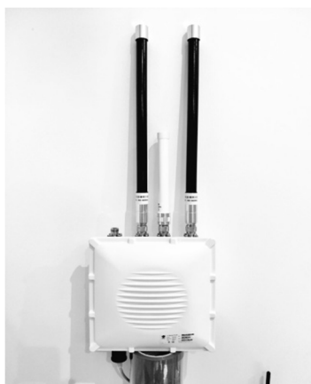
Figure 5. LoRa Outdoor Gateway RAK7249
