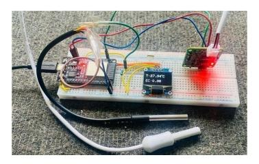
TEST CASE 1- The temperature sensor will show the room temperature. When the TDS Sensor is dry andnot exposed to air,it will show an EC value as zero. You can view these data on OLED Screen.
