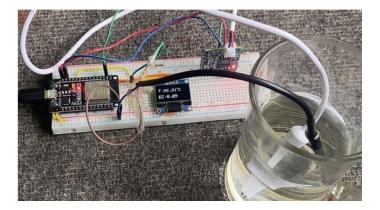
TEST CASE 2-When the temperature Sensor & TDS Sensor is dipped in water, the OLED will display the EC & Temperature value of the water.
