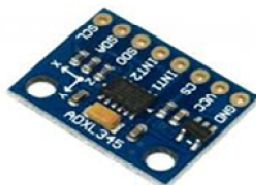
Fig.4. ADXL345 (Vibration Sensor).
