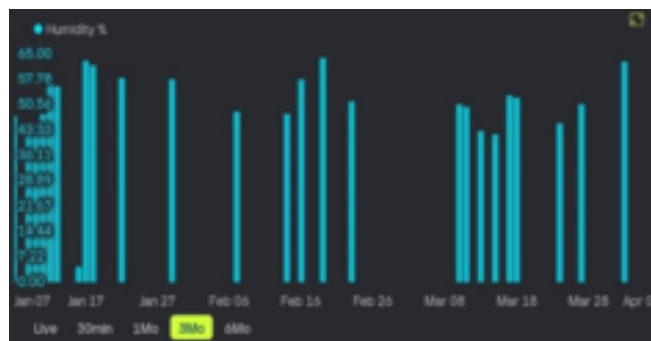
Figure 12: Three-month humidity readings graph from the DHT22 sensor.
