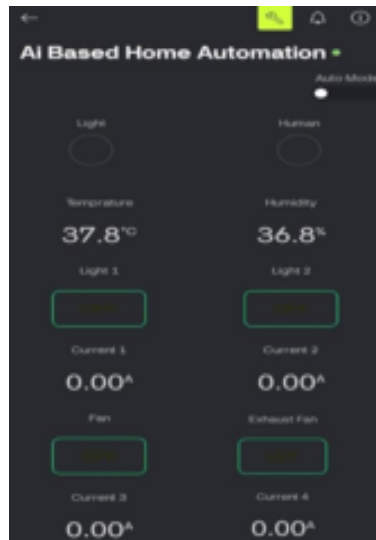
Figure 4: Blynk dashboard when the system operating while Auto Mode is off
