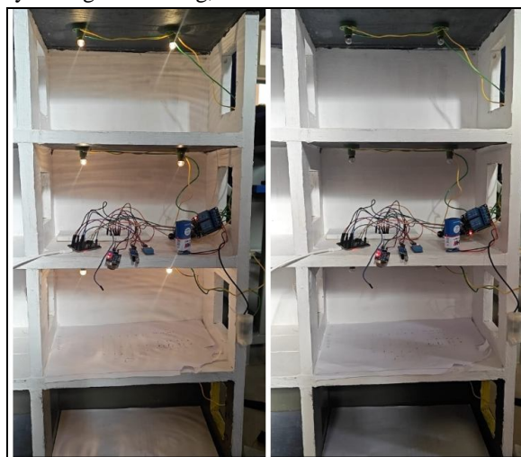
Fig. 3 Normal Supply Load Conditions (Left) Under Fire Conditions (Right)
