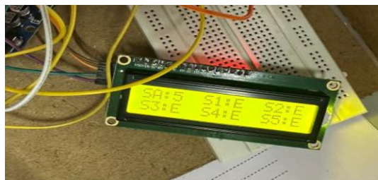
Fig 5: LCD Screen With Status Of Each Slot
