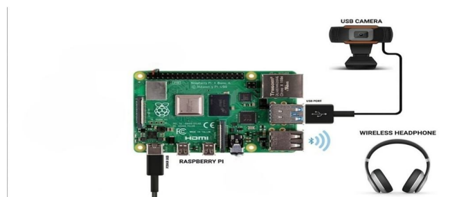
Fig. 2. Circuit diagram of the proposed smart glasses system
