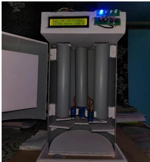
Fig.7 The internal arrangement of the medicine dispensing unit.
