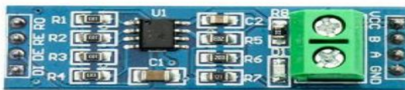
Fig. 2 Converter module for MAX485 TTL to RS485
