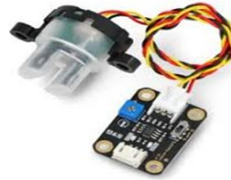
Figure 6. SEN0189 Turbidity Sensor.
