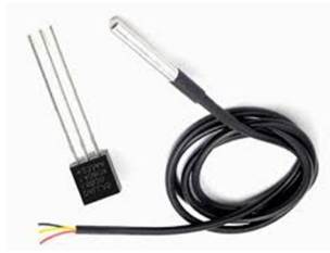
Figure 5. DS18B20 Temperature Sensor.
