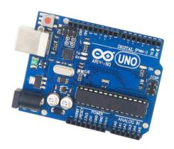
Arduino is an open-source project that created microcontroller-based kits for building digital devices and interactive objects capable of sensing and controlling physical devices. The project is based on microcontroller board designs, produced by different vendors, using different microcontrollers. These systems provide sets of digital and analog input/output (I/O) pins that can interface to various expansion boards (termed shields) and other circuits.
