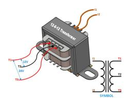
It is a chassis mounting mains transformer. Transformer consists of 240V primary windings and a center tapped secondary winding. The transformer has insulated connecting leads. The Transformer acts as a step down transformer that reduces AC power supply of 240V to - 12V. Electromagnetic induction produces an electromotive force in a conductor that is exposed to time-varying magnetic fields. Transformers are used in step up or step down of alternating voltages in power supply applications.
