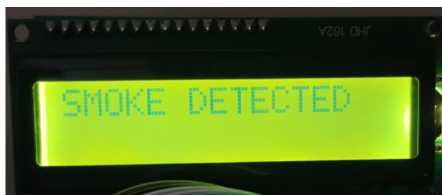
Figure 5.LCD Alert (Smoke Detected)
