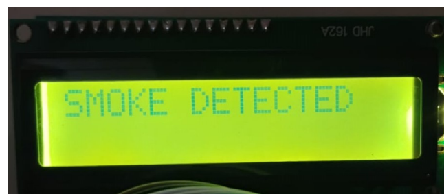
Figure 5.LCD Alert (Smoke Detected)
