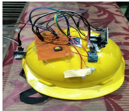
Fig. 5. Smart Tracking and Worker Safety Helmet
