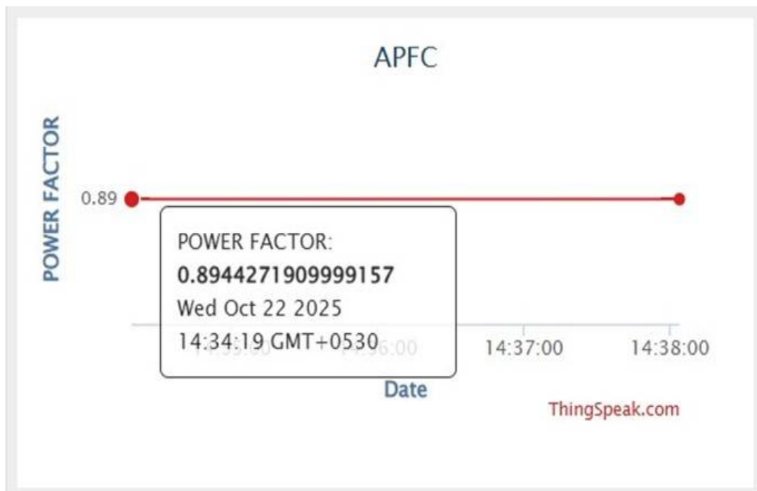
Figure 4.2: Power factor monitoring on ThingSpeak dashboard before correction.
