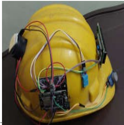
FIG: 4Safety helmet completely embedded with sensors
