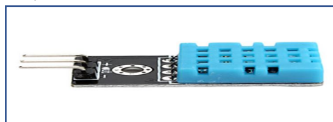
Fig: -4 DHT11 Humidity Temperature and Sensor
