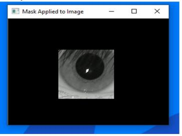
5) Segmented Output: Iris segmented from the classified output.
