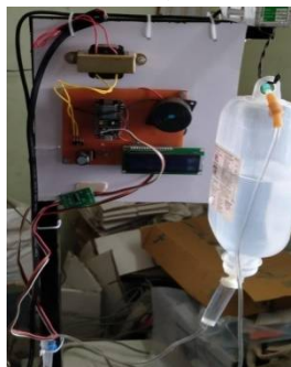
Fig. 2: Prototype of IV Drip Monitoring and Control System
