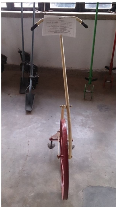
Figure 3.1. Three tyne cycle type hand hoe.
