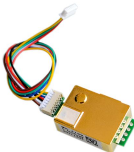
Figure 5: MH-Z19 infrared CO 2 sensor
