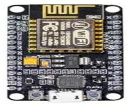
The NodeMCU (Node MicroController Unit) is an open-source software and hardware development environment built around an inexpensive System-on-a-Chip (SoC) called the ESP8266. The ESP8266, designed and manufactured by Espressif Systems, contains the crucial elements of a computer: CPU, RAM, networking (WiFi), and even a modern operating system and SDK. That makes it an excellent choice for Internet of Things (IoT) projects of all kinds.
