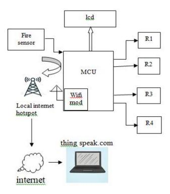
In this system, we are going to make a laboratory automation system using ESP8266 Wi-Fi module. With the help of these modules, we will be able to control lights, electric fan and other home appliances through a Wi-Fi application using our Android Smart phone. All the appliances will be connected to relays, which are controlled by the microcontroller. ESP8266 and microcontroller together act as a web Server and it will send control commands through the mobile application i.e., android software.
