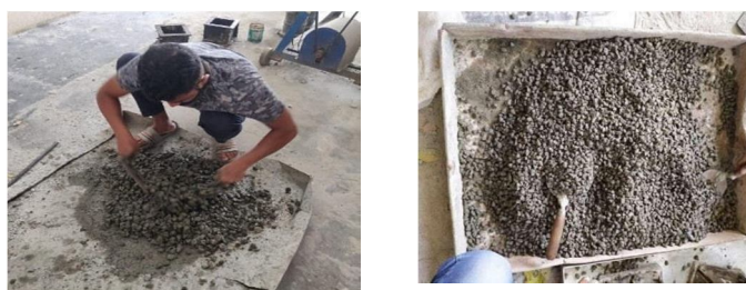
Figure 3.1 : Mixing of Pervious Concrete
