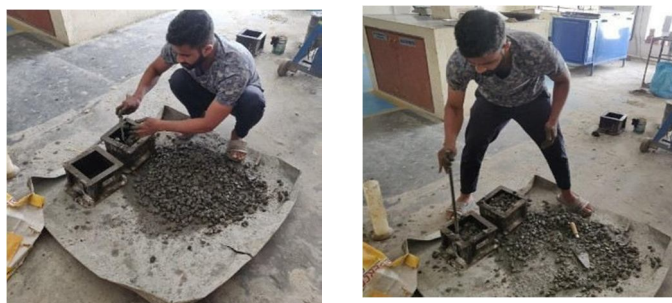
Figure 3.2 : Compaction of Pervious Concrete
