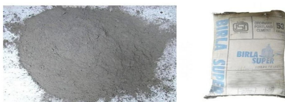
Figure 2.1: Ordinary Portland Cement of 53 grade used for the Study
