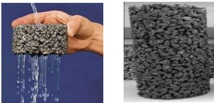
Figure 1.1 : Pervious Concrete Specimens
