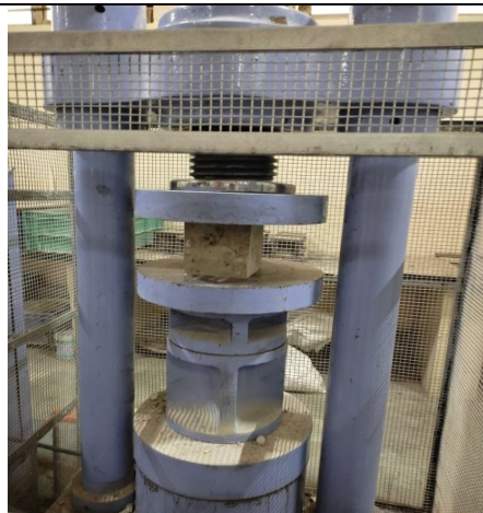
Fig 4(c) Testing of Samples for Compression in Compression Testing Machine
