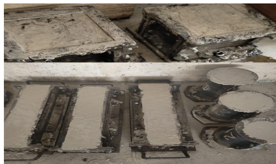
Fig 4(b) Casting of Test Specimens
