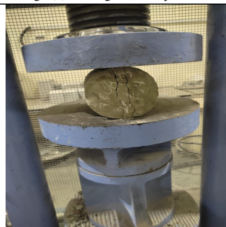
Fig 4(d) Testing of Samples for Tension in Compression Testing Machine
