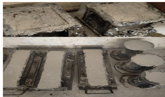
Fig 4(b) Casting of Test Specimens
