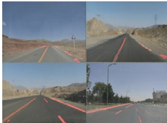
Fig. 10: The result of our lane detection on our test data
