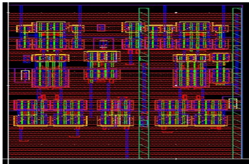
Fig.13: Layout of 2-4 decoders
