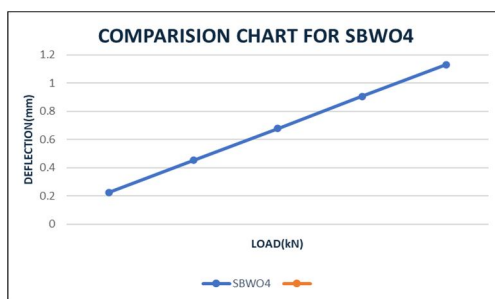
fig.5.c) Load vs Deflection curve for SBWO4
