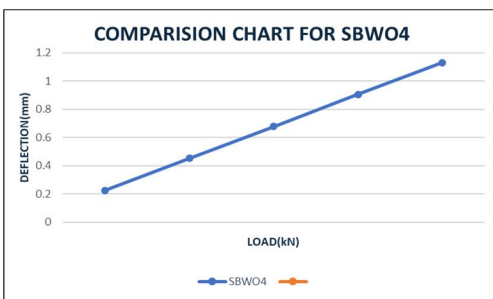
fig.5.c) Load vs Deflection curve for SBWO4
