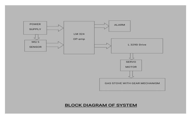
First the LPG is detected by the MQ5 sensor, and this sensed input is sent to pin no. 3 of LM324 (op-amplifier) and the output of LM324 goes to buzzer from pin no.1 as well as to pin no.2 of L293D drive. And from D drive to regulator (REES52) which will convert 5v to 1.2v and send to motor and motor rotate the gear which automatically rotate the knob of the regulator.
