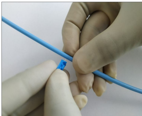
Figure.05 Manual punching process
