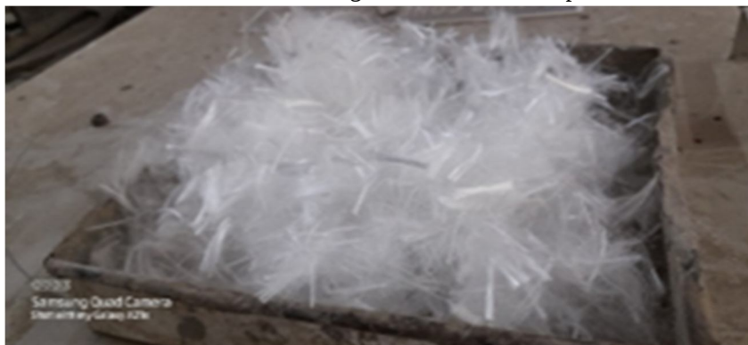
Fig. 3: 24mm monofilament polypropylene fibre
