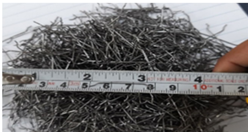
Fig. 2: End hooked steel fibre
