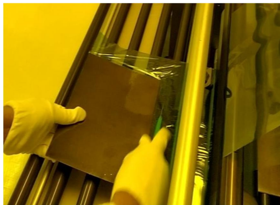
Fig.3. Dry Film Lamination
